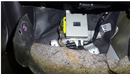
Figure 3 - Factory ECU is now ready for removal.
