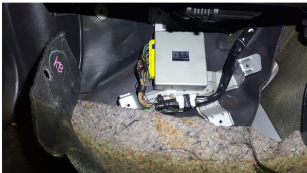
Figure 3 - Factory ECU is now ready for removal.
