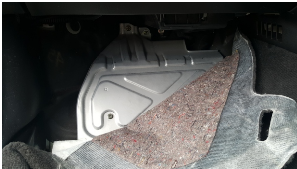
Figure 2 - Remove the panel by removing 4 nuts using a 10mm socket.
