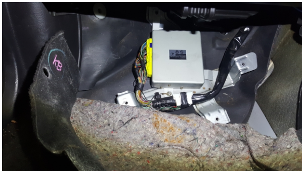
Figure 2 - Factory ECU is now ready for removal.
